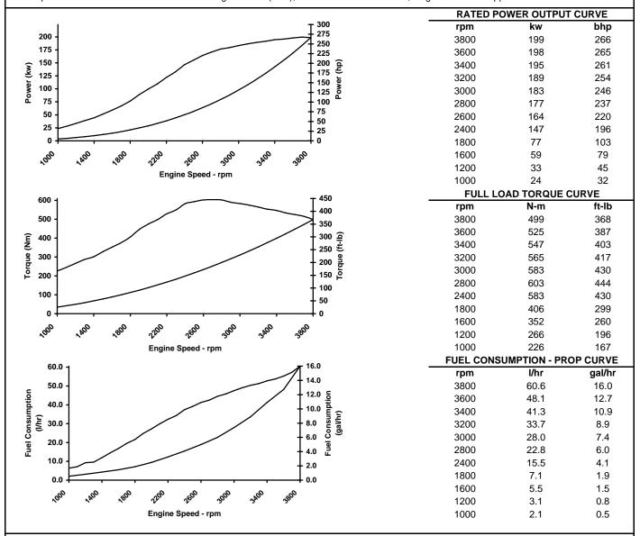
Rated Conditions: Ratings are based upon ISO 15550 reference conditions; air pressure of 100 kPa [29.612 in Hg], air temperature 25deg. C [77 deg. F] and 30% relative humidy. Power is in accordance with IMCI procedure. Member NMMA.
